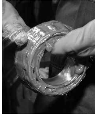
Fig. 23. Grease can easily be packed by hand.
